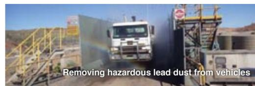
Removing hazardous lead dust from vehicles
